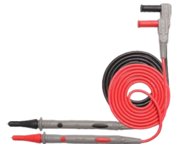
H3006 Probe:Length 130mm,TipΦ4mm Banana Plug:Φ4mm 90 degree bend plug Wire:18AWG,red/black Length:1200mm Safety Class:EN61010-031,1000V CATIII/600V CATIV,MAX 10A
