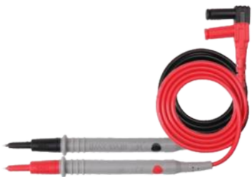
H3001 Probe:Length 130mm,TipΦ2mm Plug:Φ4mm 90 degree bend plug Wire:20AWG,red/black Length:1000mm Safety Class:EN61010-031,1000V CATIII/600V CATIV,MAX 10A
