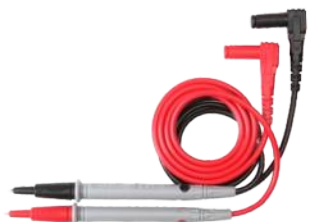
H3001 Probe:Length 130mm,TipΦ2mm Plug:Φ4mm 90 degree bend plug Wire:20AWG,red/black Length:1000mm Safety Class:EN61010-031,1000V CATIII/600V CATIV,MAX 10A
