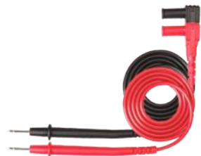
H3004 Probe:Length 90mm ,TipΦ2mm Plug:Φ4mm 90 degree bend plug Wire:24WG,red/black Length:800mm Safety Class:EN61010-031,1000V CATII
